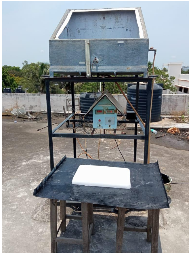
Fig 4.10 Photograph of solar still with wooden tetrahedrons
