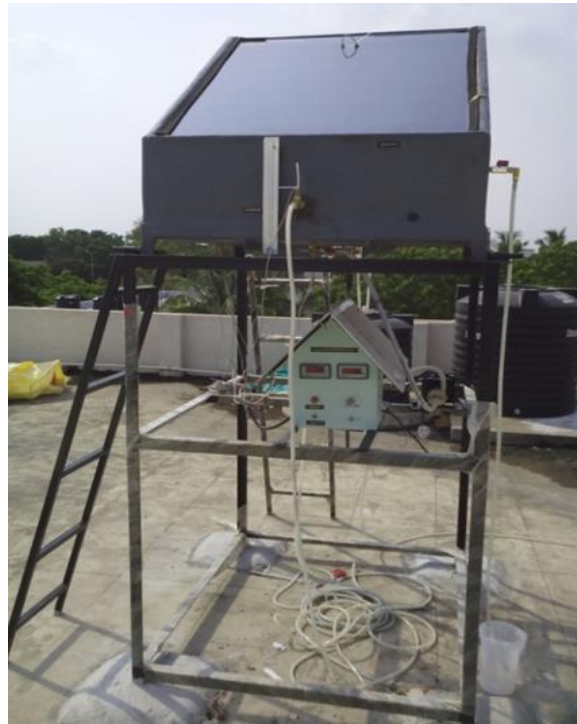
Figure 1b: Photograph of the working solar still.
