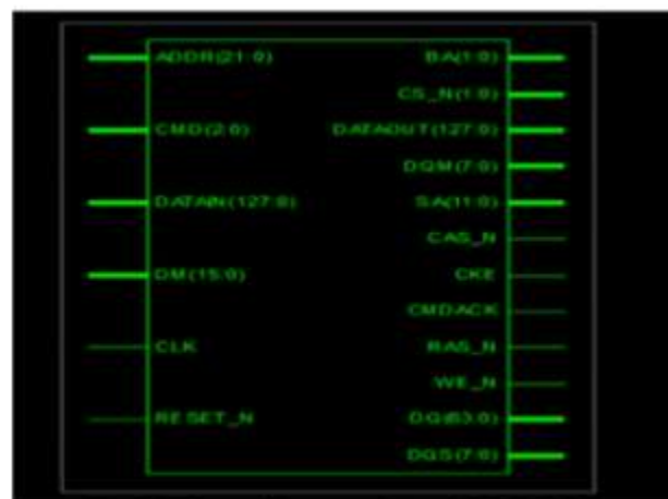
Figure 2: RTL schematic of DDR Controller
