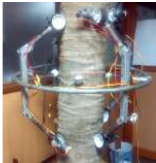
Figure 12. Pole Climbing Robot in Action
