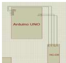
Figure 5. Circuit diagram of connecting bluetooth module with arduino.
