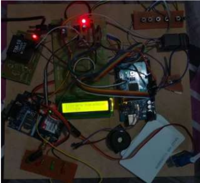
Fig 4: Hardware setup of RFID library management system
