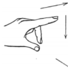
Fig 3.6 Fleming's Left Hand Rule
