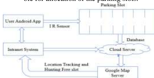
Fig. 3:- Parking Architecture using IR sensor
