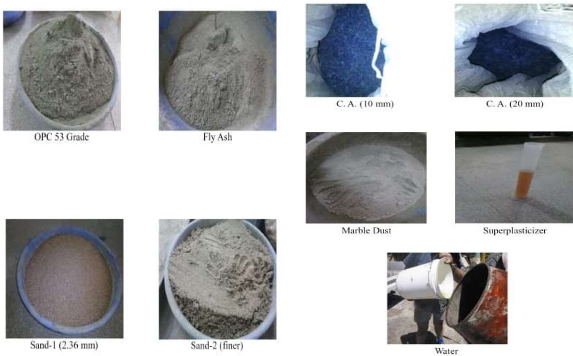
Fig 1. Ingredients of High Strength Concrete
