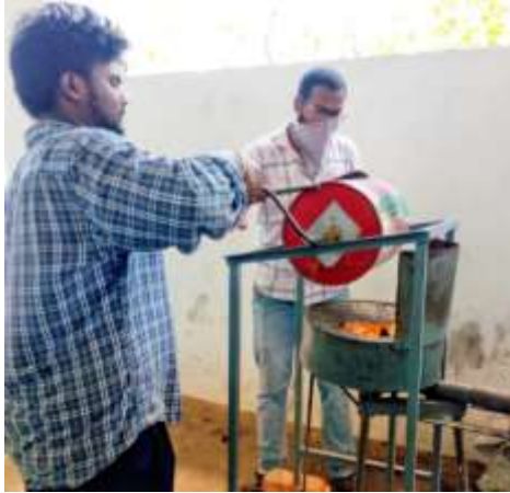
Fig 1 Wet Mixing Of Sand with ‘HA’
