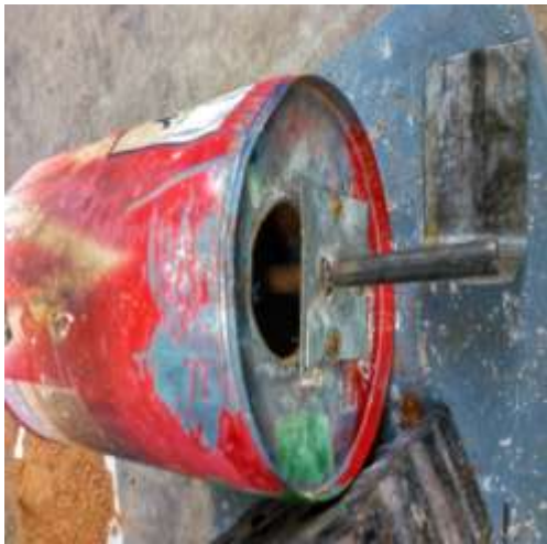
Fig 2 C-Drum for wet mixing
