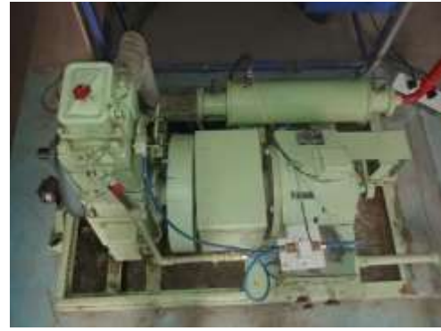
Figure 6 &7 Computerized Diesel Engine set up
