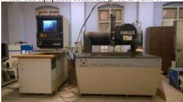
Fig. 2. Photograph of the AWJM setup at Anna University
