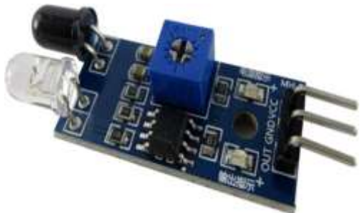
Figure 8: IR proximity sensor
